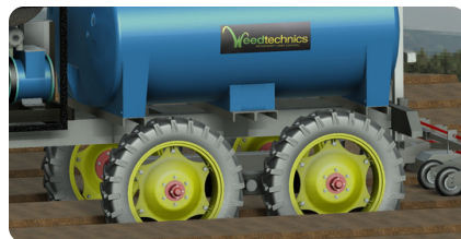
High clearance wheels available as option for deep wheel furrow grow-beds. Ground clearance up to 500mm/20"
